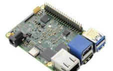
**SBC:** Single-board computers using semi-customized or fully proprietary hardware for very demanding control applications. Soft PLCs can interface with industrial I/O hardware while executing programs within commercial operating systems.
